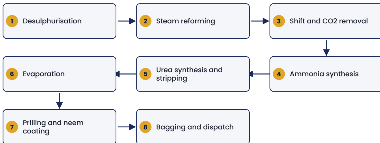
Process flow for urea from natural gas
