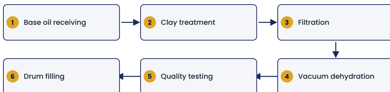
Process flow for transformer oil
