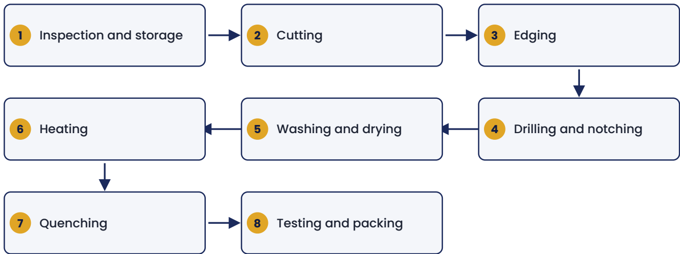
Process flow for toughened glass
