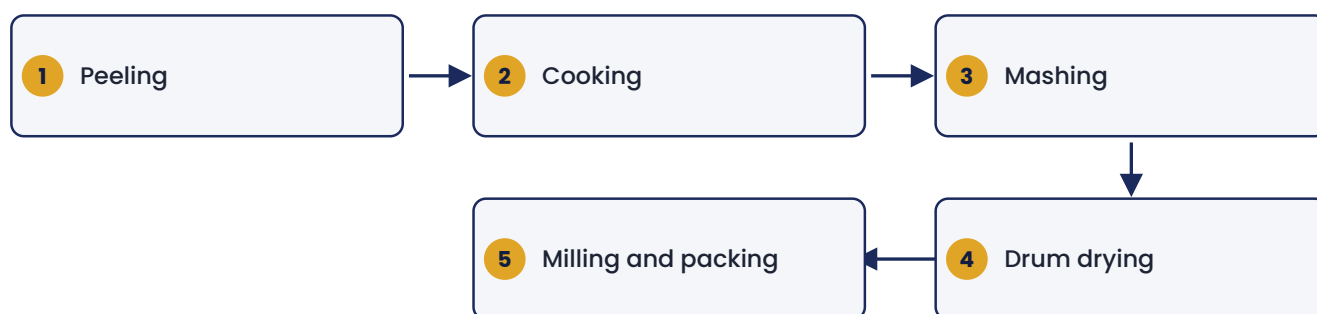
Process flow for potato flakes and powder
