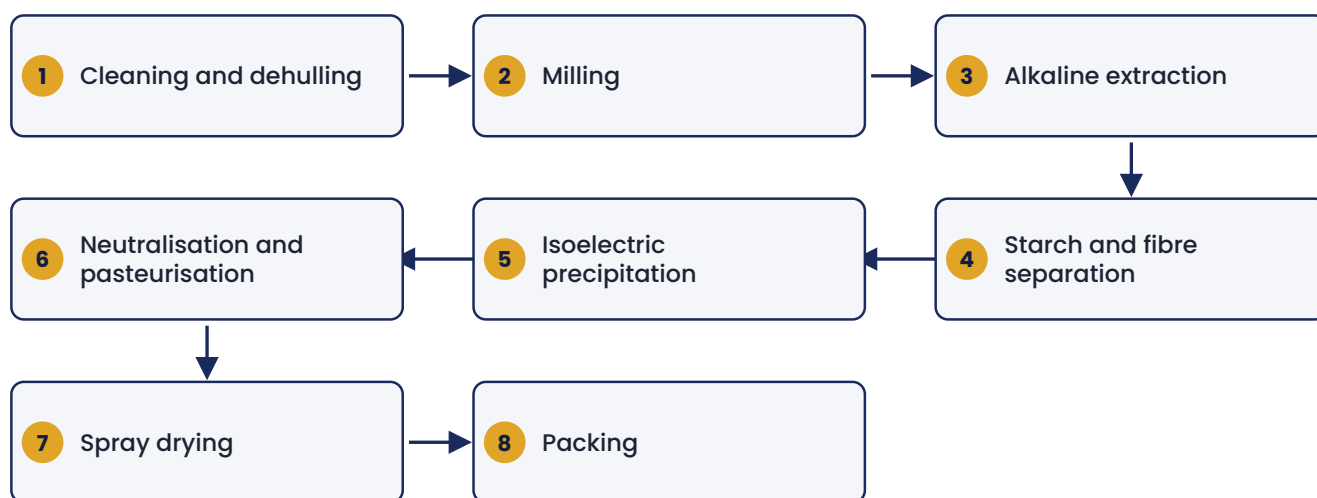
Process flow for pea protein isolate concentrate
