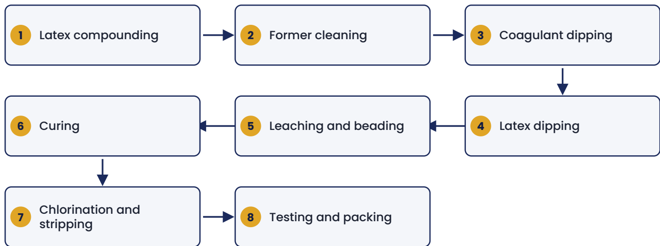
Process flow for nitrile gloves
