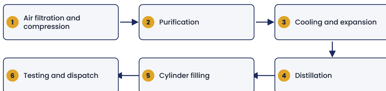
Process flow for industrial gases
