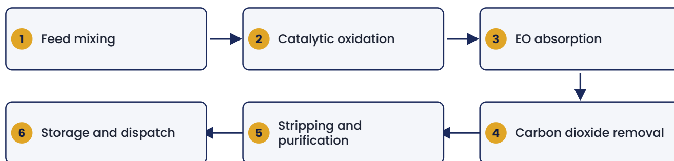
Process flow for ethylene oxide
