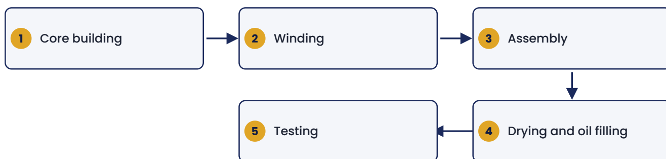
Process flow for distribution transformers
