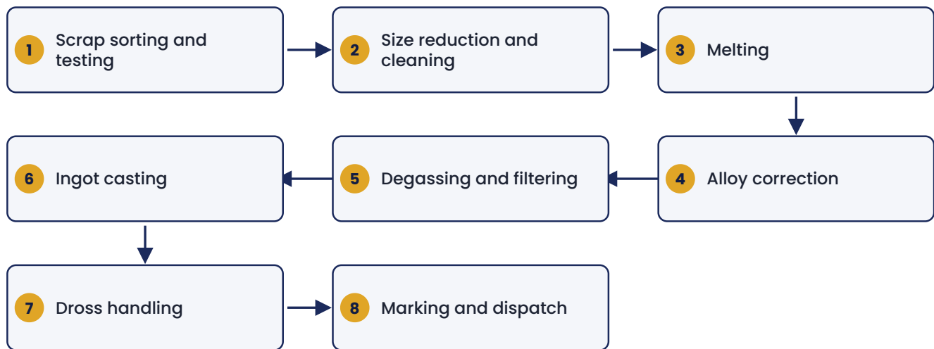
Process flow for aluminium ingot from aluminium scrap
