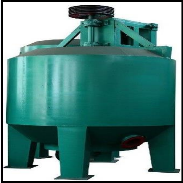
High Consistency Hydrapulper
